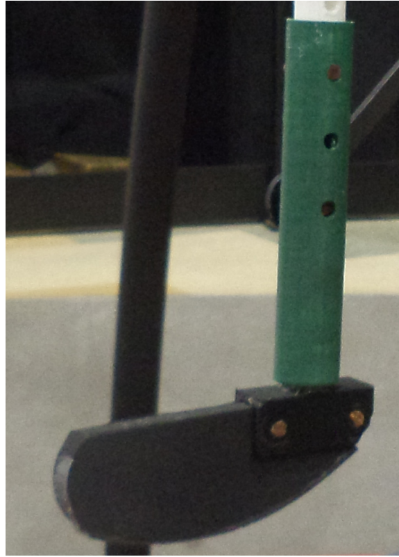
Figure 3.4: Foot, foot bracket and shin of LUIGI made with ABS
