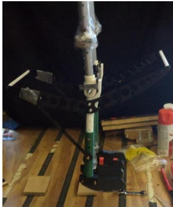
Figure 4.5: Example of the attachment of weights on LUIGI
