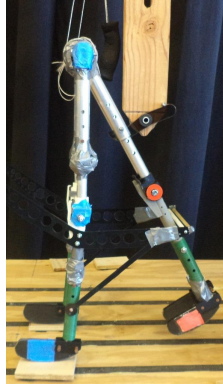
Figure 5.1: Launcher setup to remove human variability
