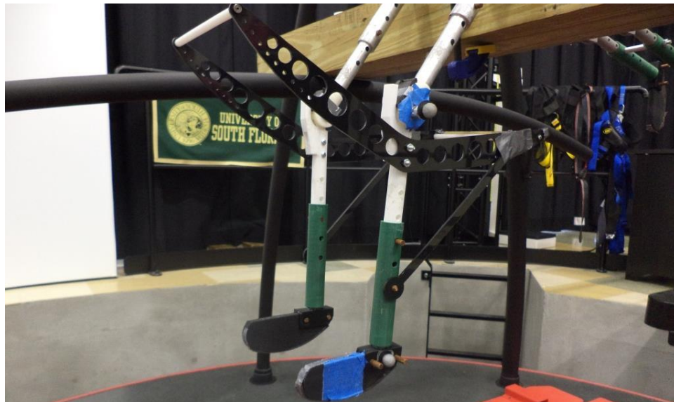
Figure 4.2: Knee damping setup on the CAREN system
